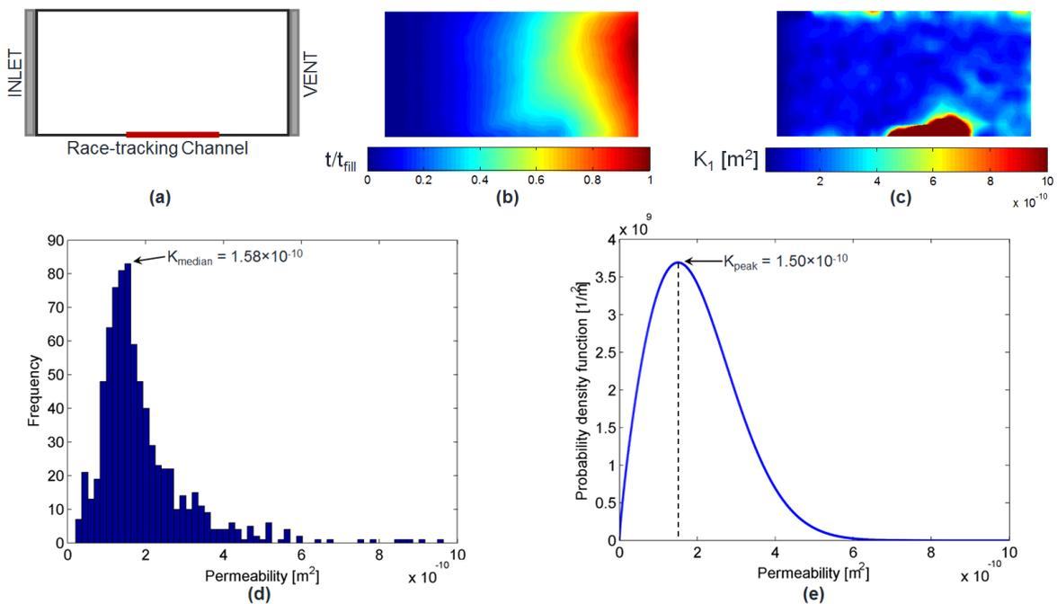
**Figure 2:** Results of an experiment with a race-tracking channel introduced intentionally. (a) Mold details, (b) flow front propagation in the experiment, (c) estimated permeability map, (d) histogram of the estimated permeability values, (e) probability density function corresponding to the histogram.
